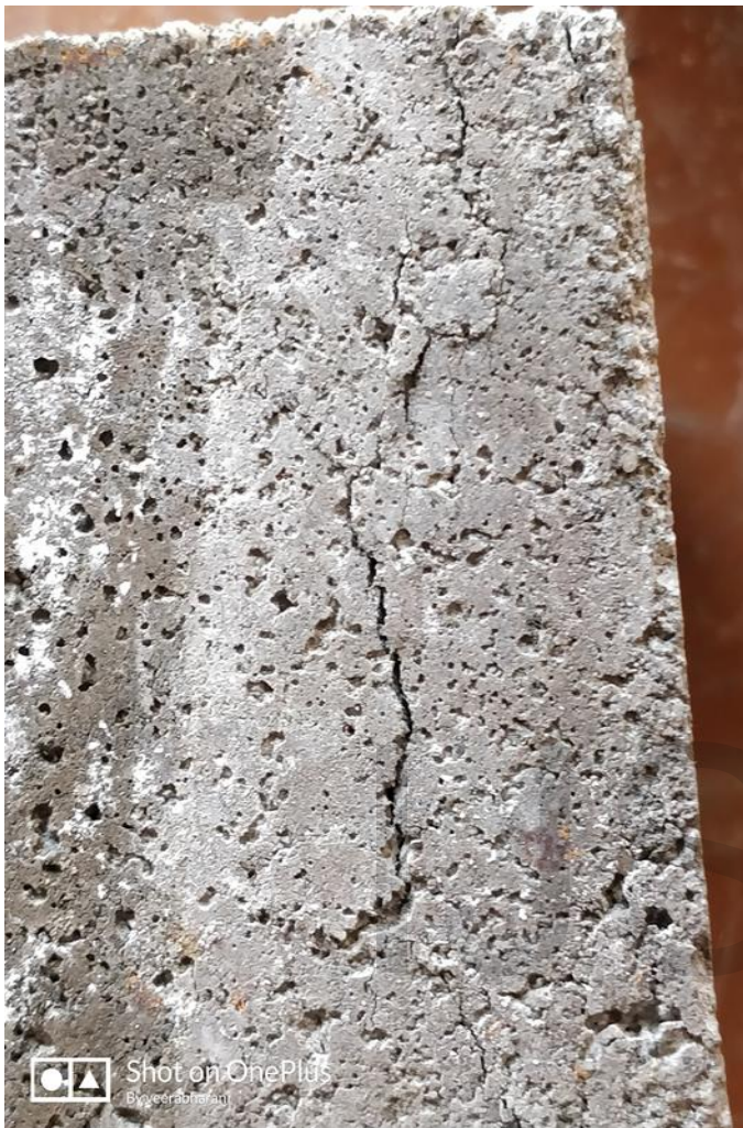
Fig 1 creation of crack by applying load using compressive machine
